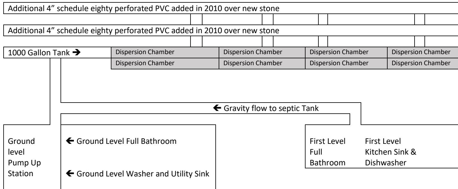
Notes: This is a diagram only and is not to any scale of measurement
